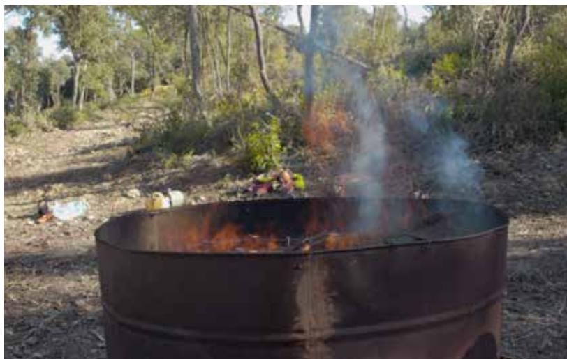
Figure 1. Transportable boiler to produce biochar directly in the forest. Photo: AV Video.
