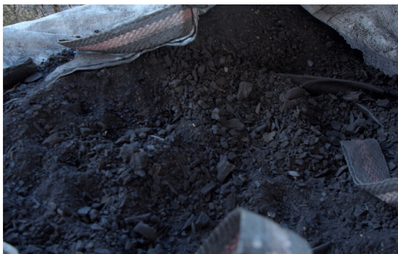
Figure 2. Biochar sample obtained by the pyrolysis of plant biomass. Photo: AV Video
